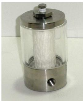
The filter is a standard 2.5 and several different grades of filter elements are available. The filter has an 1/8" port and an 1/4" NPT in and out. It is also available in an 1/8" NPT in and out.
